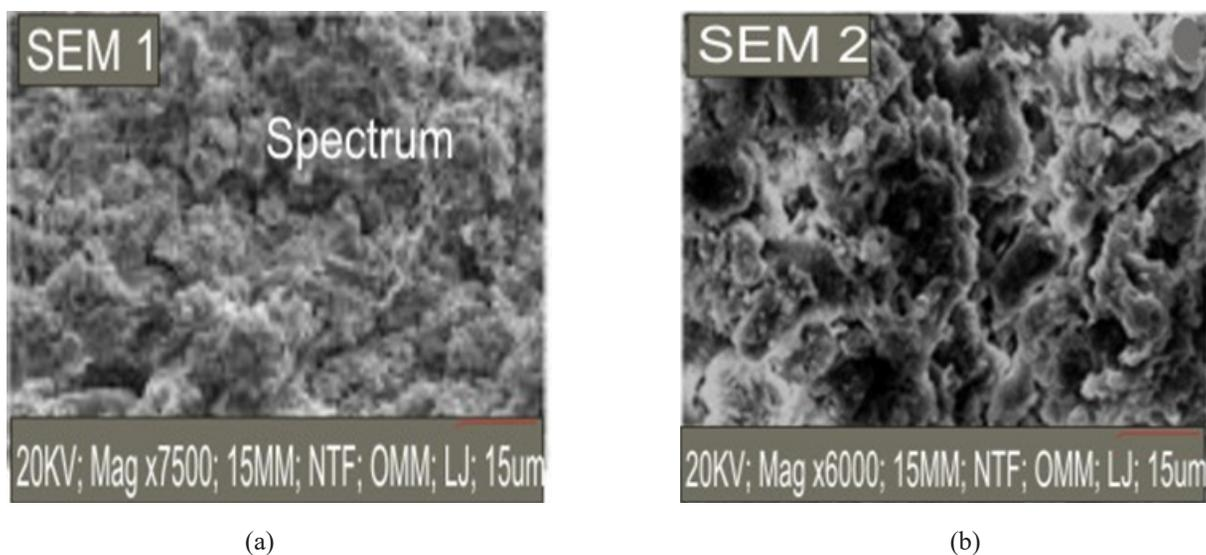
Fig. 2. SEM images of (a) raw and (b) calcined anthill.
