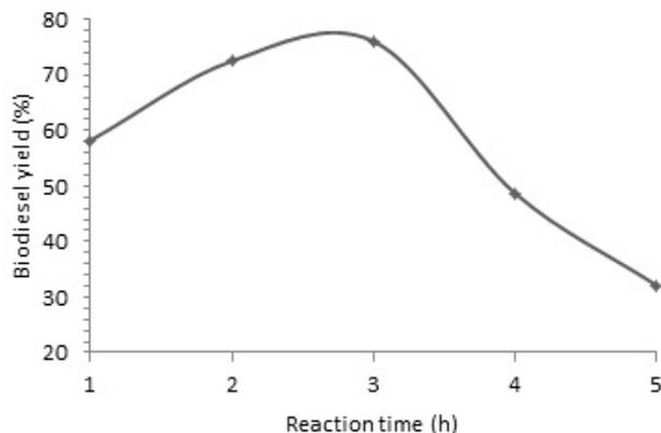
Fig. 5. Biodiesel yields at different reaction time at fixed reaction temperature = 70°C, catalyst dose = 2.0 wt. % and methanol/oil molar ratio of 6:1.
