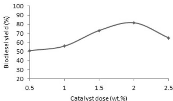
Fig. 6. Biodiesel yields at different catalyst doses at fixed reaction temperature = 70°C, reaction time = 3 h and methanol/oil molar ratio of 6:1.
