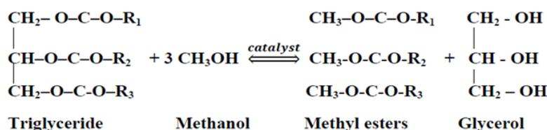
Fig. 1. Transesterification of oil with methanol.
