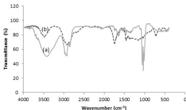
Fig. 7. FTIR spectra of (a) palm olein oil and (b) palm olein oil biodiesel.
