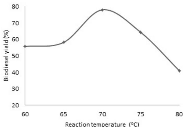
Fig. 4. Biodiesel yields at different reaction temperatures at fixed reaction time = 3 h, catalyst dose = 2.0 wt. % and methanol/oil molar ratio of 6:1.
