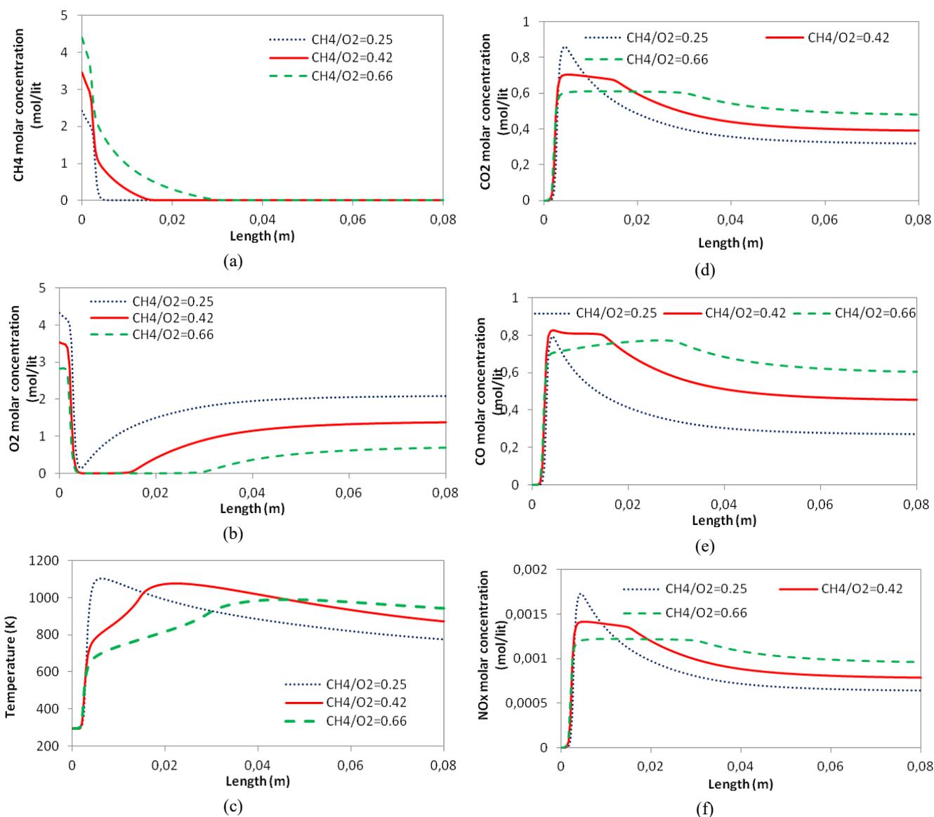
Fig. 3. An effect of the fuel/air ratio on (a) the methane concentration profile, (b) the oxygen concentration profile, (c) the temperature profile, (d) the carbon dioxide concentration profile, (e) the carbon monoxide concentration profile, (f) NOx concentration profile.
