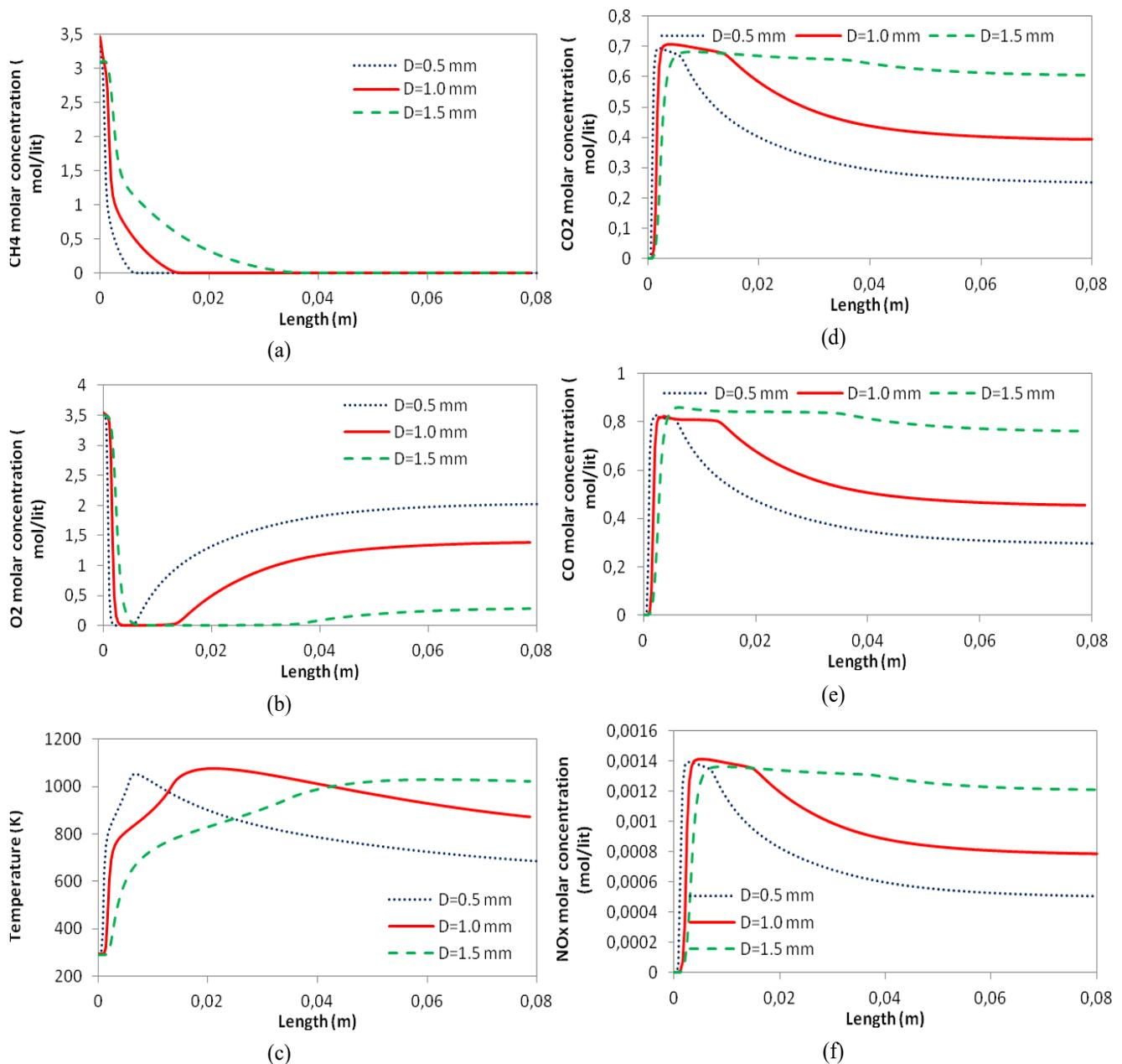
Fig. 2. An effect of the orifice diameter change on (a) the methane concentration profile, (b) the oxygen concentration profile, (c) the temperature profile, (d) the carbon dioxide concentration profile, (e) the carbon monoxide concentration profile, (f) NO<sub>x</sub> concentration profile.
