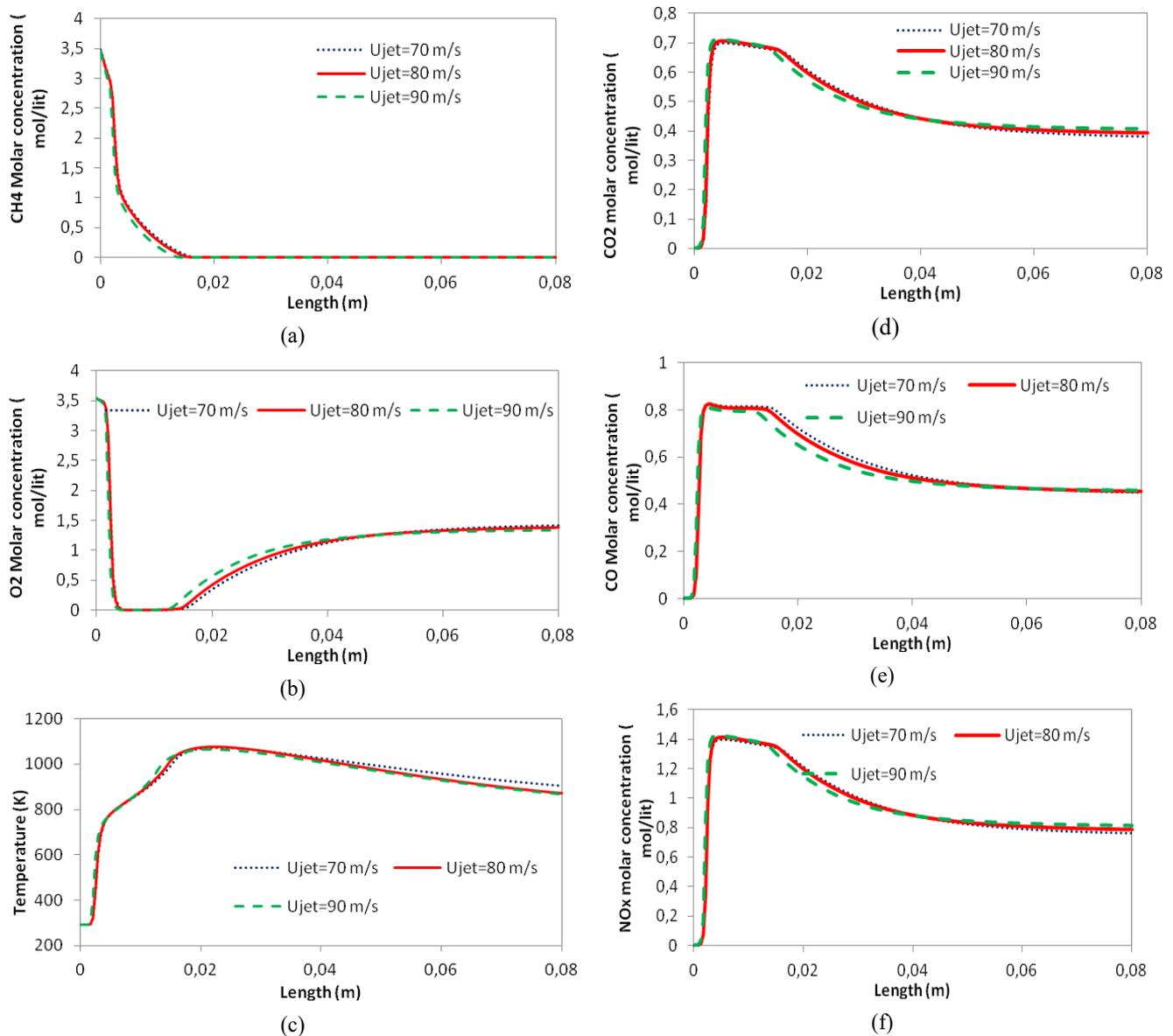
Fig. 4. An effect of the fuel jet velocity on (a) the methane concentration profile, (b) the oxygen concentration profile, (c) the temperature profile, (d) the carbon dioxide concentration profile, (e) the carbon monoxide concentration profile, (f) NOx concentration profile.
