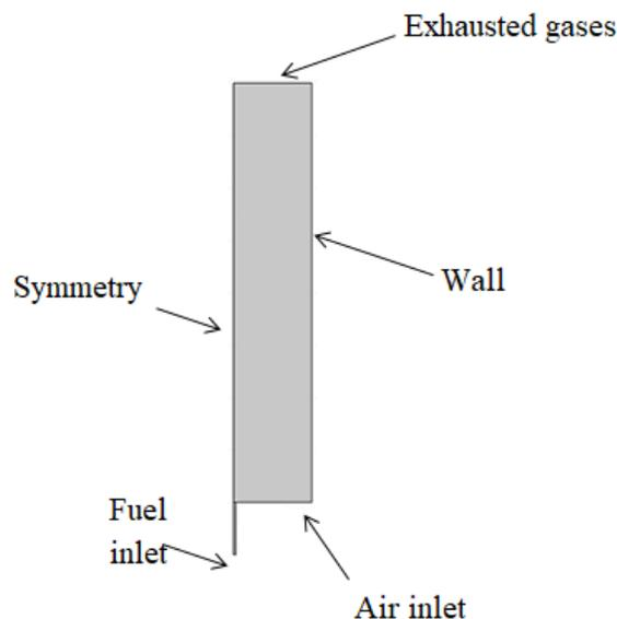
Fig. 1. Geometry and related boundary conditions of a burner.
