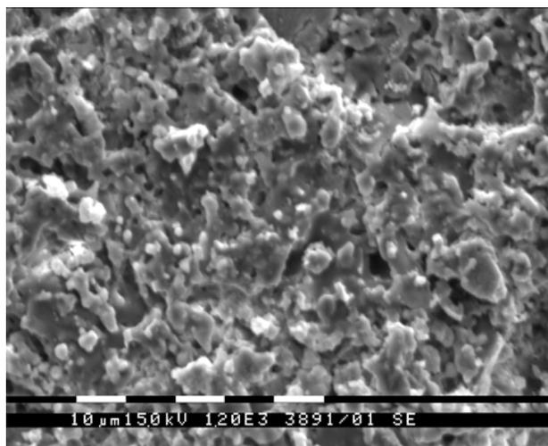
Fig. 6. SEM of sintered at 1100°C ceramic membrane with composition 3.
