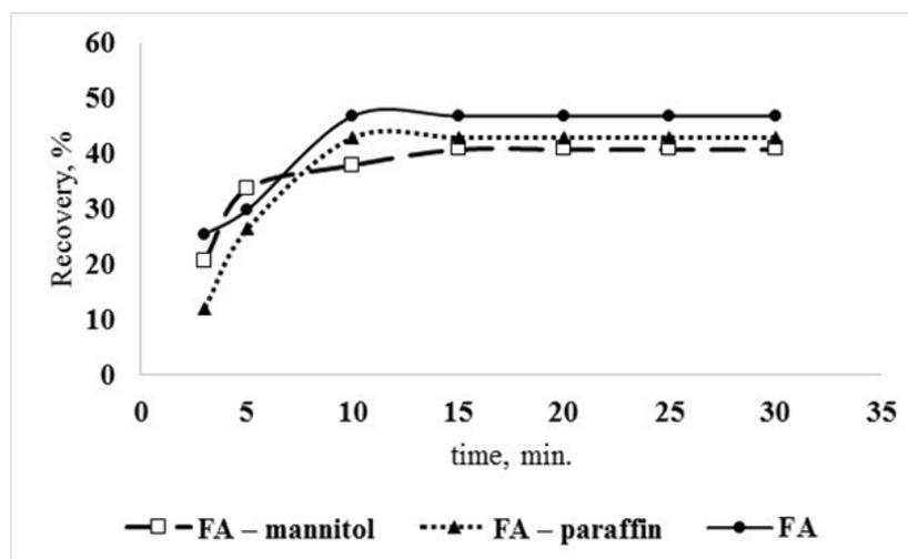
Fig. 2. Dependence of boric acid recovery on the phase contact time.
