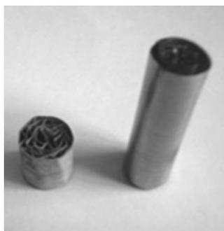
Fig. 1b. A perspective view of the metal block for the laboratory sample of catalyst.
