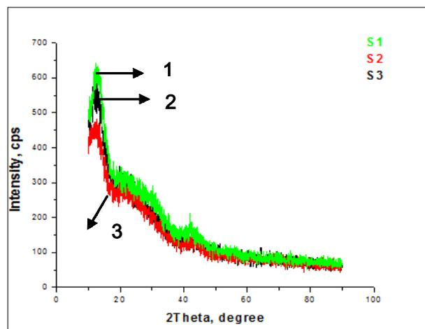
Fig. 2. XRD patterns of SBA-15 samples: S1 – sample 1, S2 – sample 2, S3 – sample 3.
