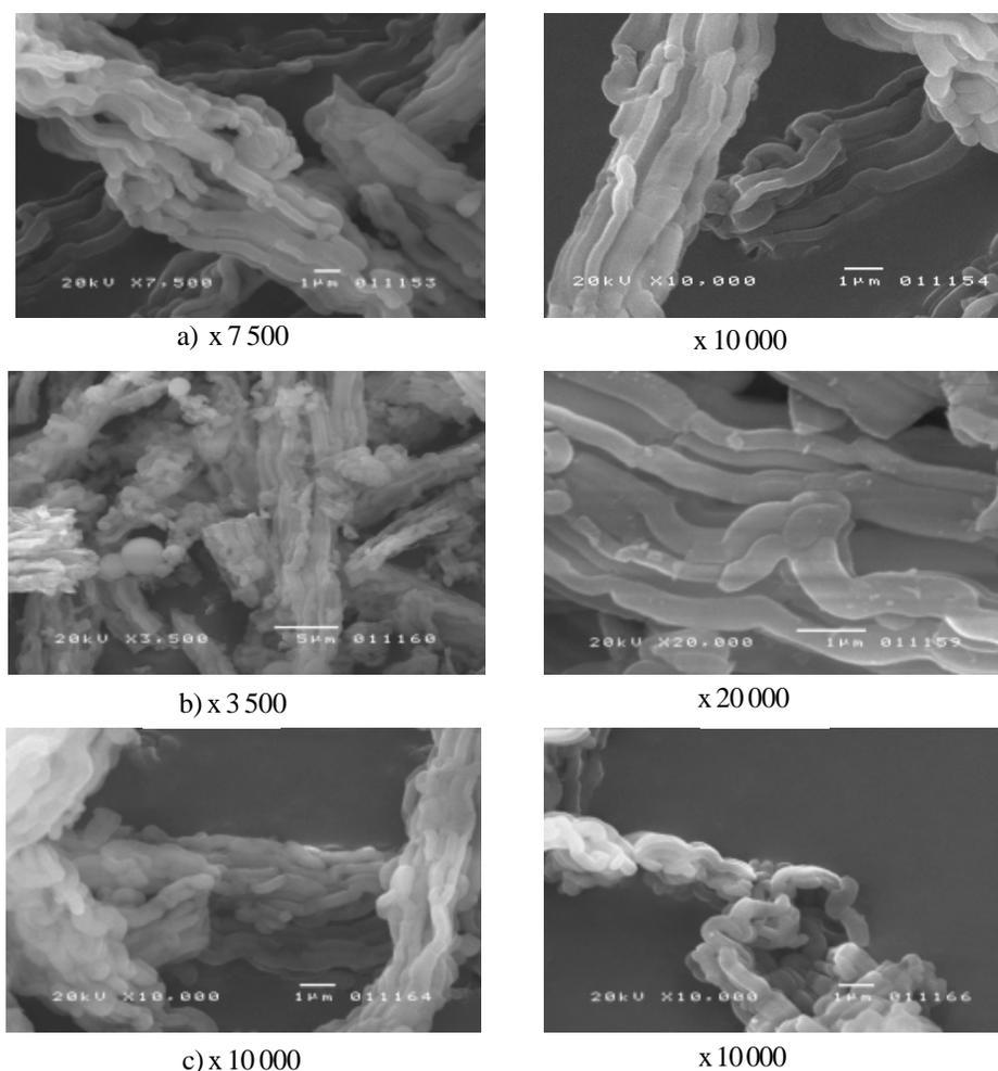
Fig. 4. SEM micrographs of SBA-15 at different magnifications: a – sample 1, b – sample 2, c – sample 3.
