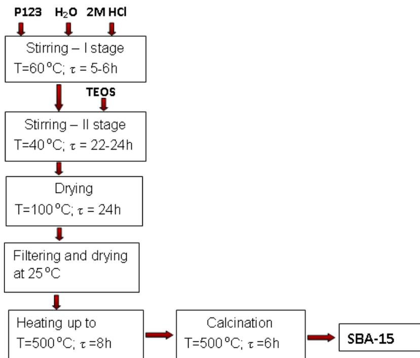
Fig. 1. Block scheme of the SBA-15 synthesis.
