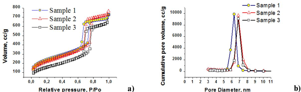
Fig. 6. Nitrogen adsorption-desorption isotherms (a) and pore size distributions (b) of SBA-15.
