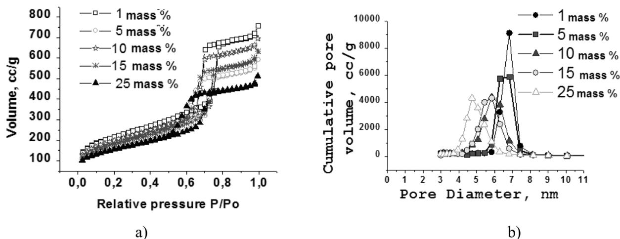
Fig. 8. Changes of the pore volume and BJH pore size distribution in the T-SBA-15 samples prepared with different content of TiO<sub>2</sub> after calcinations at 500°C.
