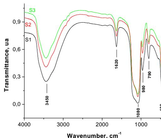
Fig. 3. FTIR spectra of SBA-15 samples.
