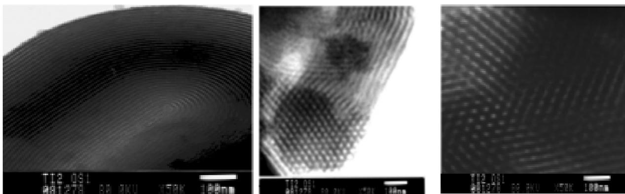
Fig. 5. TEM micrographs of a SBA-15 sample. Magnifications for all samples are  $\times$ .
