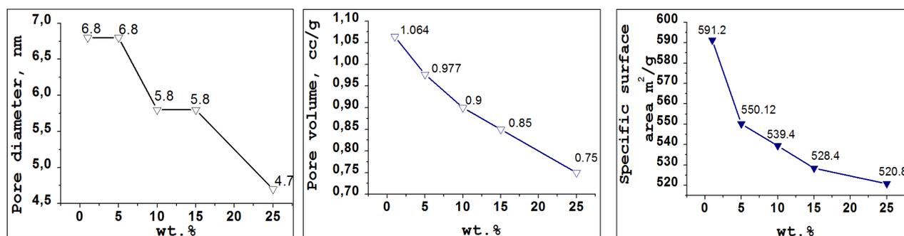
Fig. 7. Changes of the pore diameter (a), pore volume (b) and specific surface area (c) vs. mass % TiO<sub>2</sub>.
