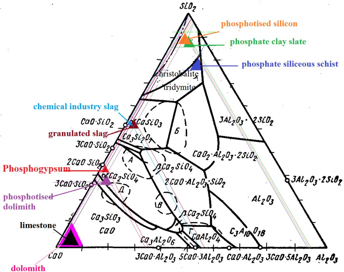
Fig. 1. Areas of technical products and wastes in system CaO - Al<sub>2</sub>O<sub>3</sub> -SiO<sub>2</sub>.
