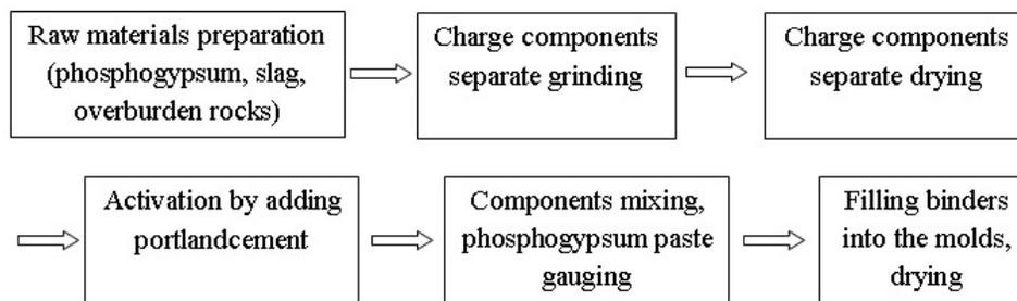
Fig. 2. Technological scheme for obtaining an unburned mineral binder.
